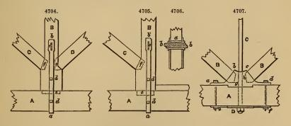
Fig. 4705 shows the queen-post. A is the tie-beam; B the post, tenoned at e; c the strut; and D the straining-piece; the strap, ba; and bolt, dd. Fig. 4707. In this figure a superior construction is shown, in which a king-bolt of iron, C D,
